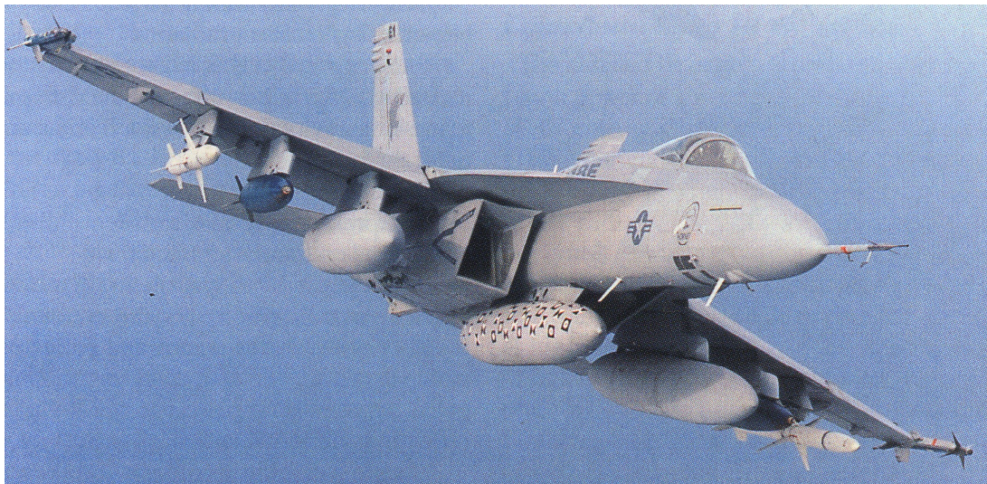
One of the developmental F/A-18E/F airframes demonstrates how certain VLO techniques can be applied to a design that is anything but stealthy to begin with: all major apertures are aligned with the wing leading and trailing edges, and the fuselage sides and air intakes are canted at the same angle as the fins. Antennae and vents are aligned with the main wing planform. The main undercarriage and engine bay doors have serrated edges. Because the air intake ducts do not provide line-of-sight blockage to the engines, they house a radar absorbent baffle which reduces intake efficiency but also decreases a major source of radar return. Photo McDonnell Douglas
