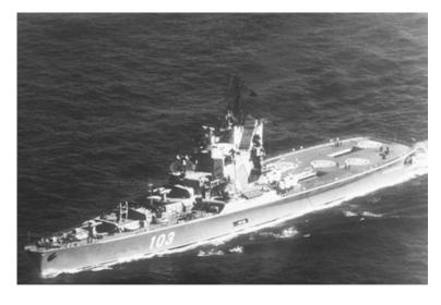
ship. The class was designed to carry 14 of the new Ka-25 antisubmarine warfare helicopters, themselves just entering service at the time.
