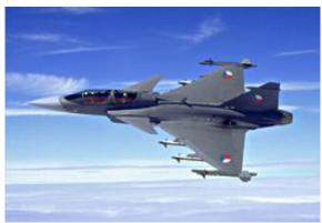
JAS-39C (2007): As JAS-39C (2006) with a new weapon, the Meteor MR-AAM. This missile replaces the RB-99 AMRAAM in most loadouts.
