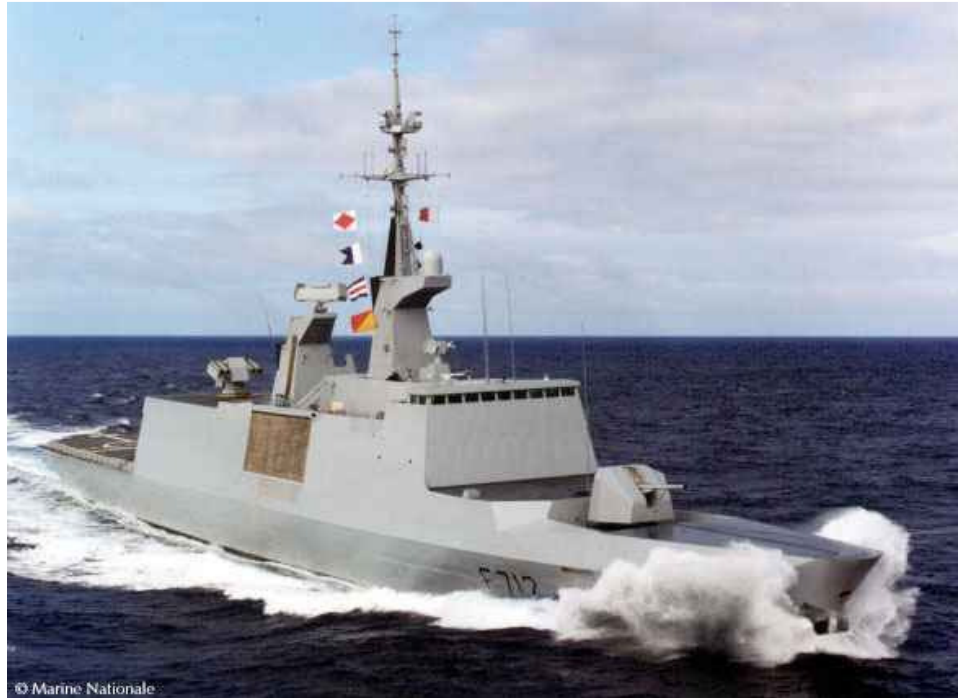
Courbet (F712) is the 3rd Lafayette-class frigates, one of which relies rather on survivability rather than on firepower. It has been designed to maintain a stealthy signature and use its AS-565 Panther (ASuW) in sea state 6.
