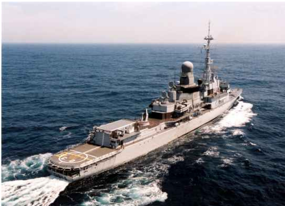
Jean-Bart (D615) is the 2nd F70 type frigate specialized in air defense for carrier. It has the most advanced communication devices like the carrier Charles de Gaulle and thus is part of her escort like brethren Cassard (D614). Both usually carry an AS 565 Panther ASuW helicopter.
