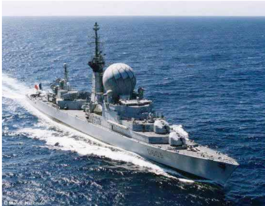
Duquesne (D603) belongs to a former air defense class of frigates and serves now as a training ship. It will be replaced by the first Horizon-class destroyer by 2008. Fitted with the last Masurca (MARitime SURface Contre avions – Naval SAM against aircrafts) in service in the Marine Nationale, Duquesne is used as an escort for amphibious ships.
