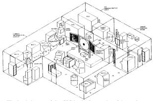
The basic layout of the CIC in the Perry-class frigate shows clearly the US tendency to concentrate all the major subsystems of the C3 system in a limited area, often in a single room.
